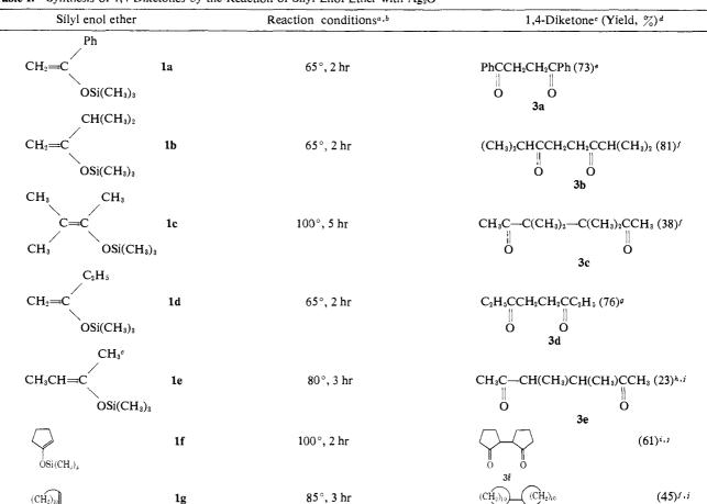
Table I. Synthesis of 1,4-Diketones by the Reaction of Silyl Enol Ether with Ag<sub>2</sub>O
